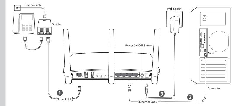
Press the power **ON/OFF** button of your modem router and make sure the LEDs (especially the ADSL LED) display as shown below.
